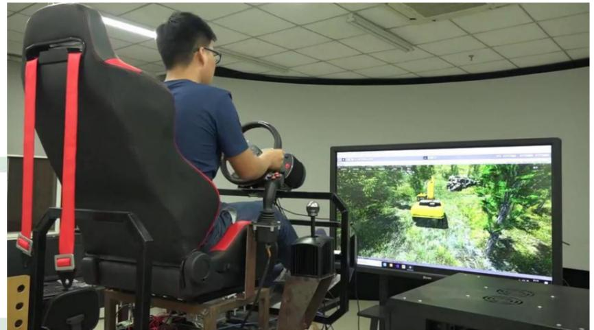
Simulated Driving Suit to Control a Virtual harvester
