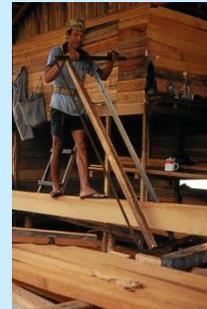
Fig. 2: Manual Plank Sawing (Indonesia)
