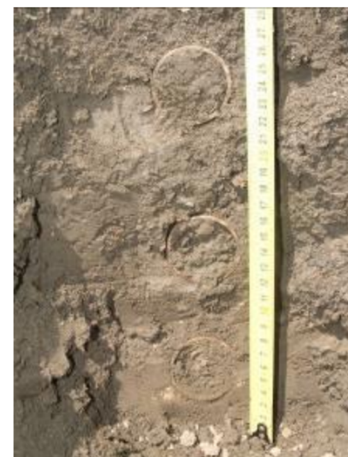
Fig. 4. Placement of the sampling rings on different depth stages
