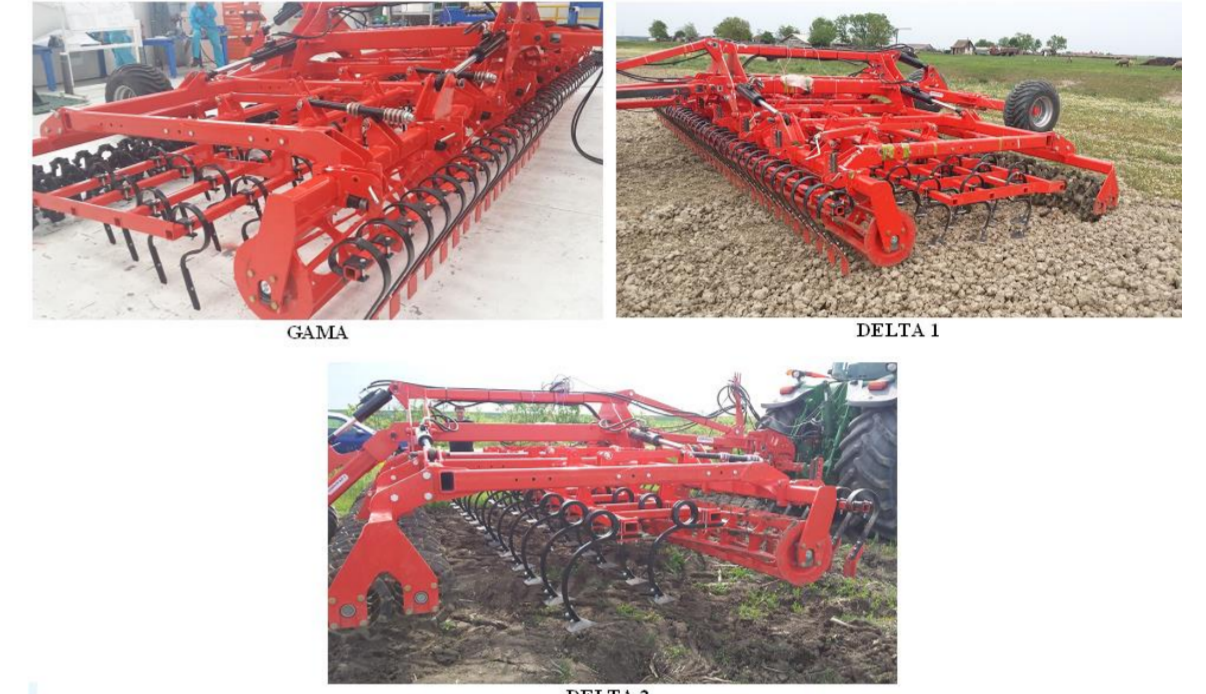
Fig. 2 The prototype vibro-combinator SANDOKAN 2 equipped with the three types of active elements (GAMMA, DELTA1, DELTA2)
