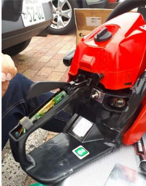
Figure 2. Sensors and the PCB was installed inside the handle grip.
