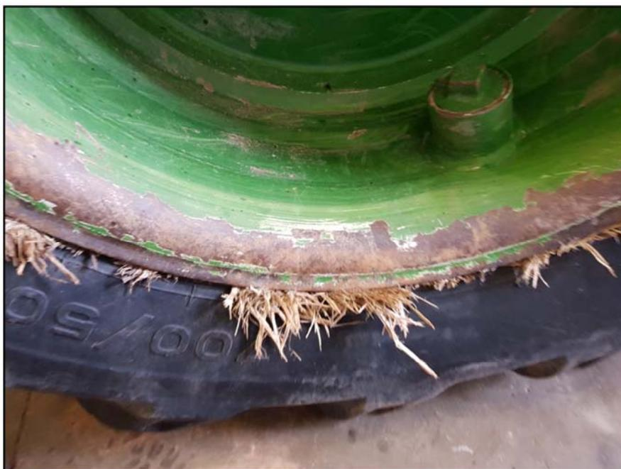
branches can slide between the rim flange and the tyre, see Fig. 6. Especially wooden splinters can be pressed with high forces against the rim flanges when the wheel is side sliding against a tree stump.
