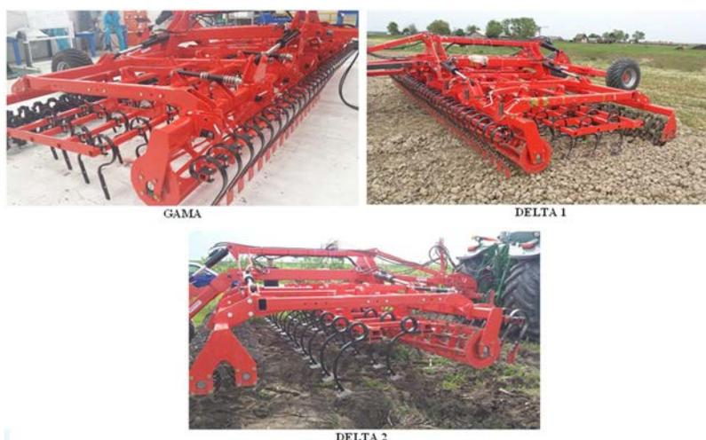
**Fig. 3** The prototype vibro-combinator SANDOKAN 2 equipped with the three types of active elements (GAMMA, DELTA1, DELTA2)
