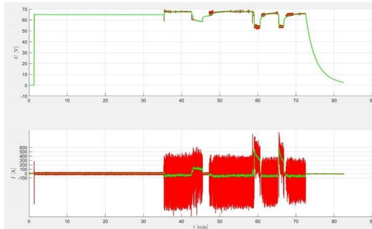
**Fig. 5 - Battery current and voltage measured during the trailer operation cycle**
