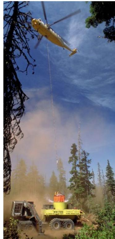
*Image 4 - A helicopter transfers water to a super-skidgine for night shift work*
