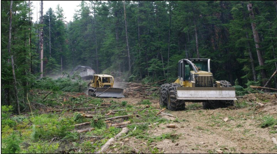
*Image 1 - Cutting indirect fireline with feller-buncher, while track and wheel skidders swing logs to decking area*
