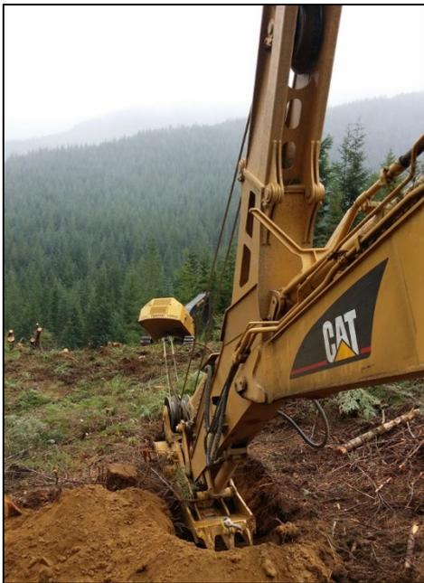
*Image 8 - Dual cable tethering system with leveling feller-buncher and remote-controlled drum set mounted on an excavator*
