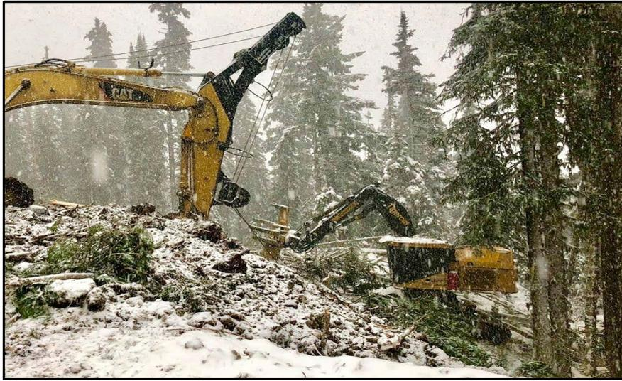
Figure 4. Tractionline winch-assist and Tigercat L870C feller buncher: Case Study 4
