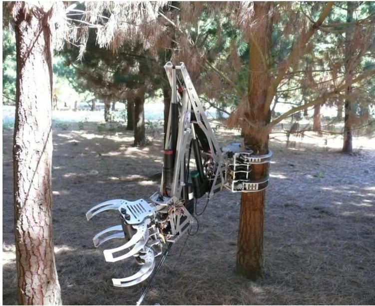
**Figure 2 Scion tree-to-tree robot platform**
