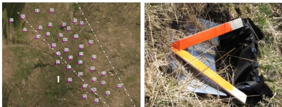
**Figure 1** Layout of the sediment traps on the 60% hillside. The dashed lines show the position of the cable corridors while the arrow indicates the downhill direction (left). Close-up of sediment trap after 2 years, the orange marker indicating the position of ground control point used in processing UAV imagery
