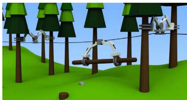
**Figure 6 Robot system to extract logs to the nearest road**
