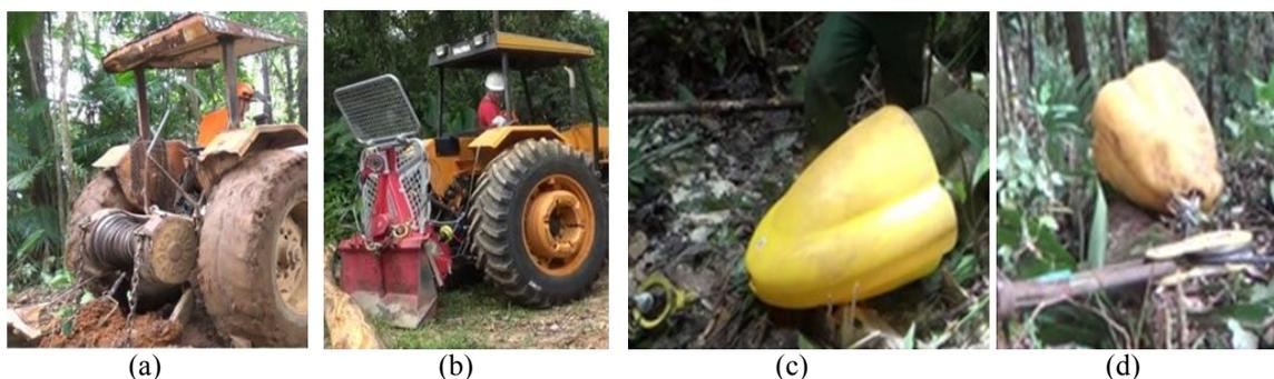
**Figure 2.** a) Tractor winch in the conventional method; b) Tractor winch in the alternative method; c) Skidding cone; d) Snatch block (Britto et al, 2017).
