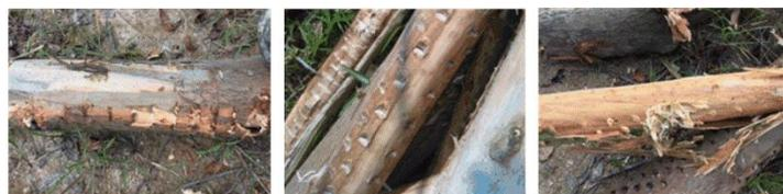
**Fig. 1** Damage to logs caused by spikes of feeding rollers
