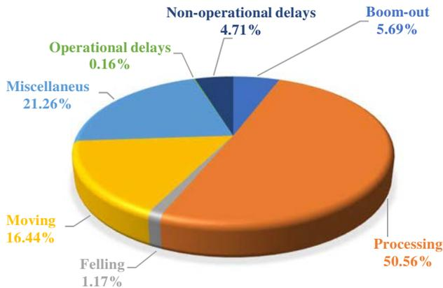
Fig. 2- Site A harvester work elements distribution
