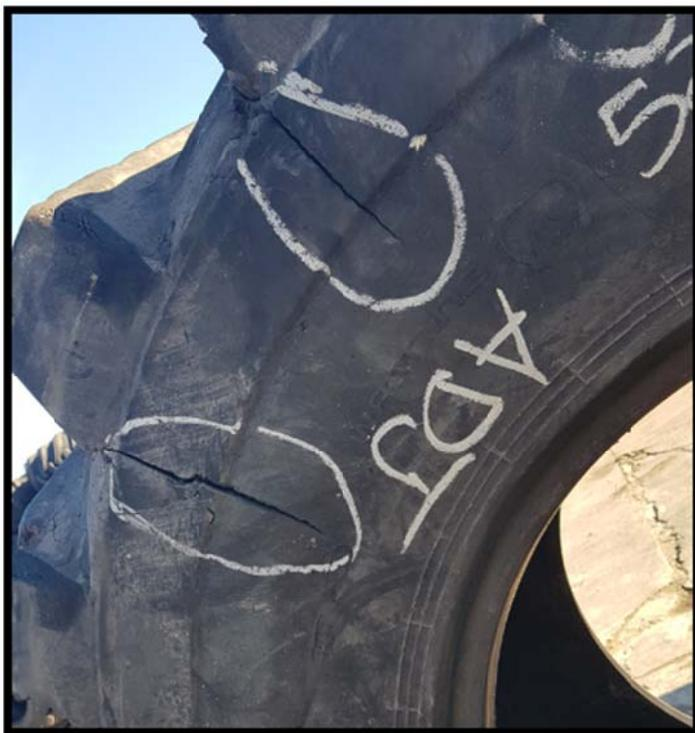
**Fig 3: Cracks caused by low inflation pressure** designer of low inflation pressure tyres.
