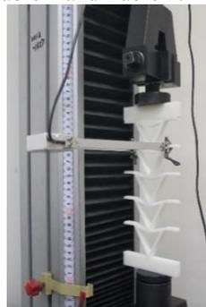
**Fig. 12 The compression experiment of V-winged NPR structure in the Y-direction**
