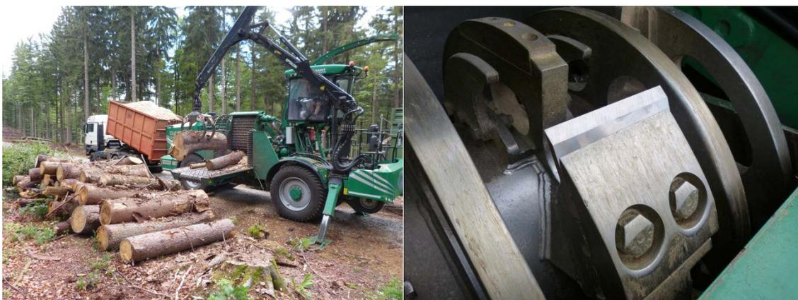
Figure 1: Chipping with the self-propelled Albach Diamant 2000 (left) was carried out with new and sharp knives (right)
