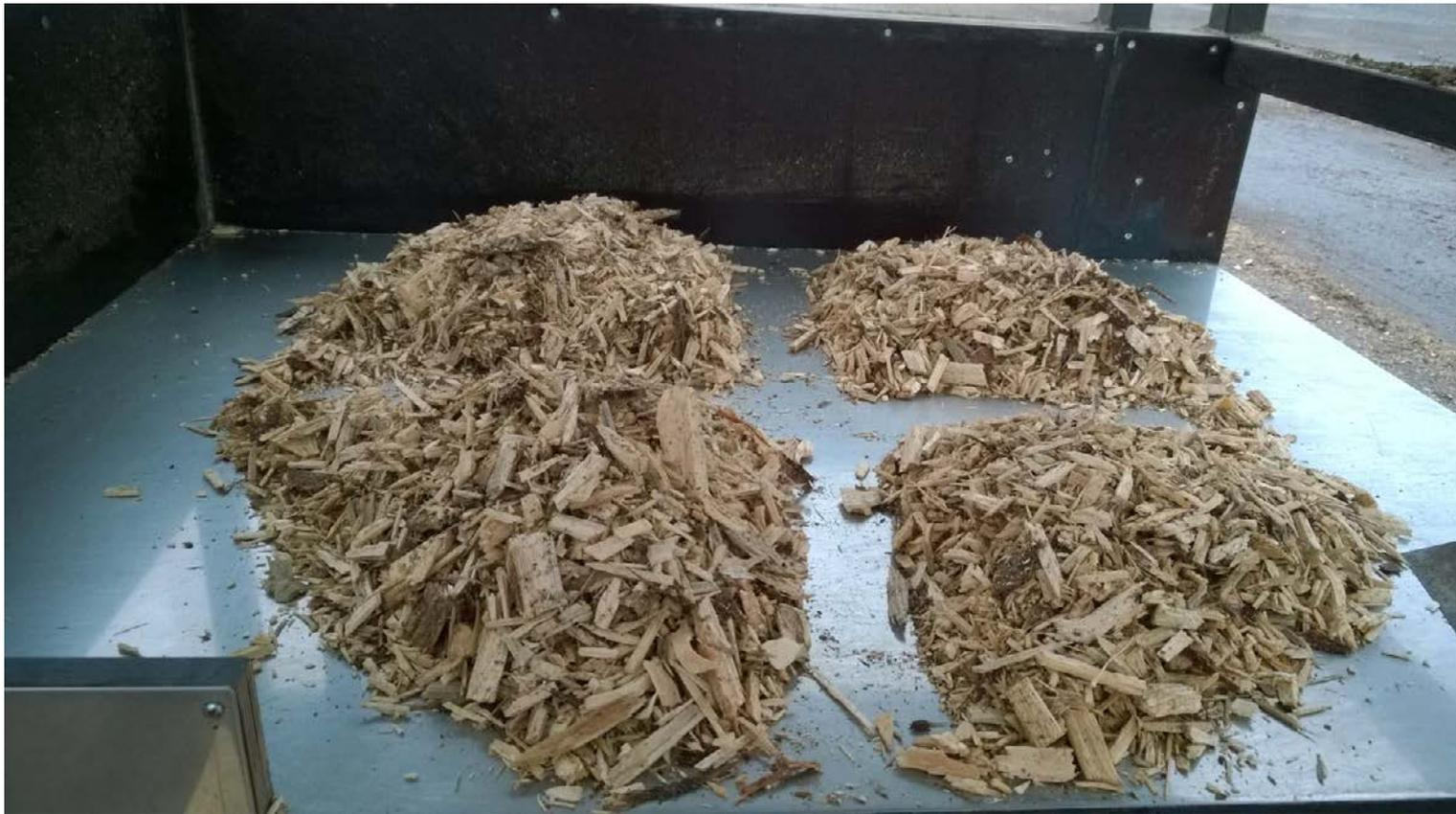
The moisture samples were taken from piled chips; 6–8 samples were taken with ladle sampling to a big plastic tub. All the samples were spilled onto a table, where chips were divided into four parts. One part was put into a duplicate plastic bag (5 litres). Plastic bags were delivered immediately to the laboratory, where the moisture content was measured using the oven dry method. The sampling method closely followed the solid biofuel standard EN 14774.
