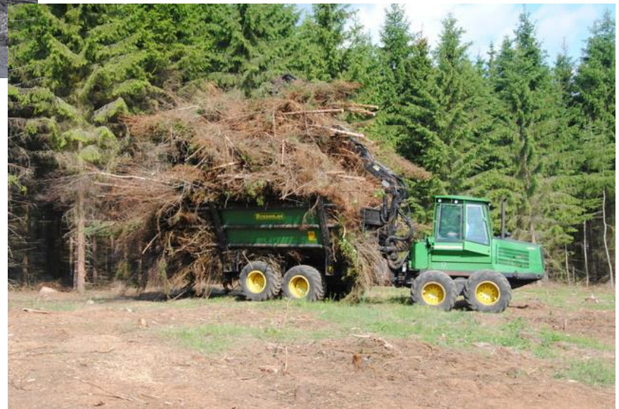
Variant 1 – forwarder with cargo of forest residues
