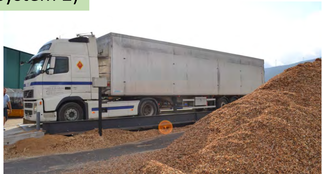
Volvo 480 truck with walking floor trailer of 90 m 3 cycle time of 3 hours and 20 minutes
