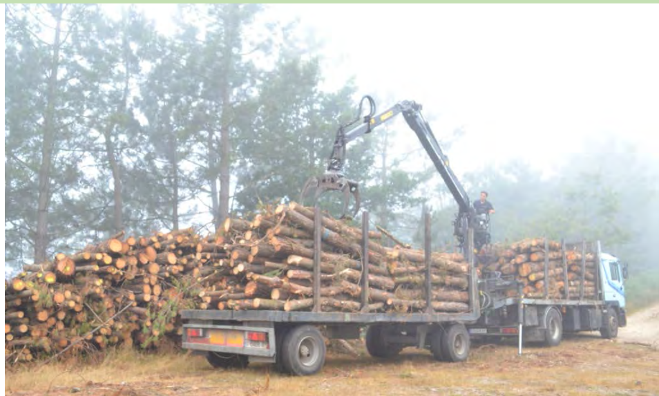
Man 19-362 truck. 24 tonnes Cycle time 3 hours and 46 minutes
