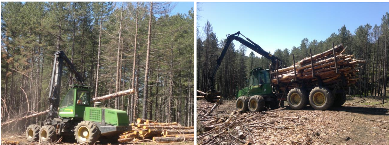
Fig. 1. John Deere 1270D harvester and John Deere 1110D forwarder in working process
