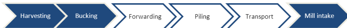
Figure 1: Process chain in German CTL systems. The unfilled cells of the processes Forwarding, Piling and Transport symbolize the lack of automatic data generation for process control and show room for optimization in the wood supply chain.
