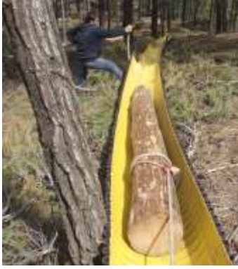
Figure 3. Controlled Sliding of the Wood-Based Products at Downhill Slope by Mobile Winch
