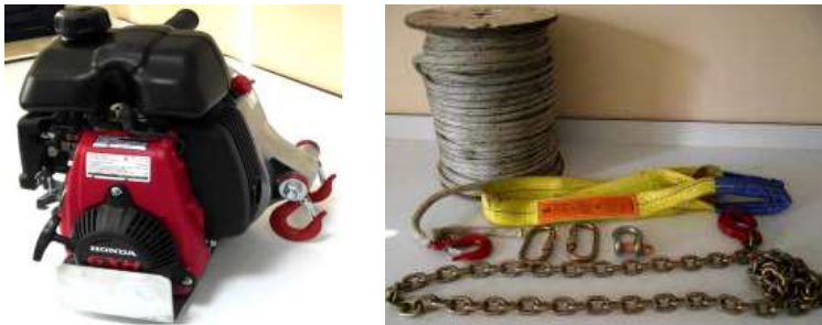
Figure 1. Mobile winch, synthetic rope and other system equipment
