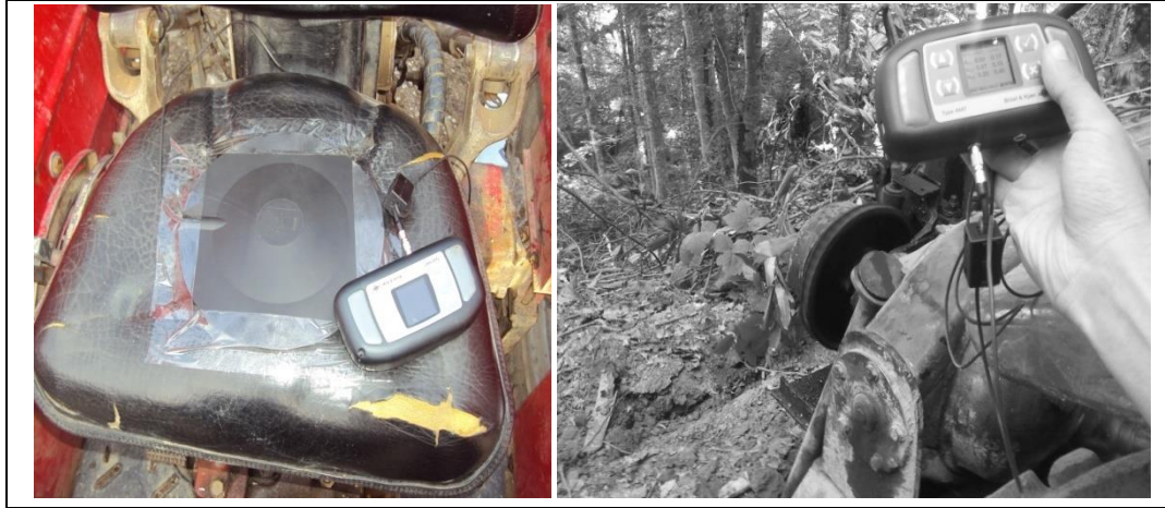
Figure 2. Brüel & Kjaer 4447 vibration measurement device with measurements to be made.
