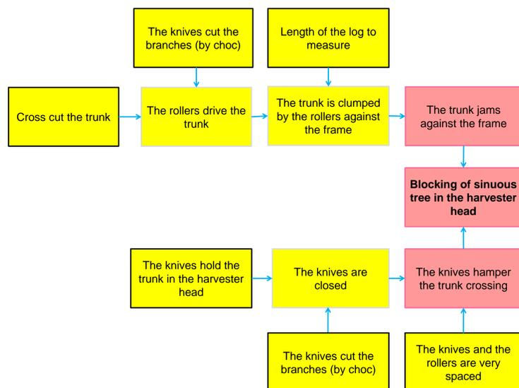
Cause-effect model of the problem "blocking of sinuous tree in the harvester head"
