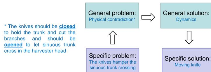
The TRIZ principle and its illustration for the identified problem "blocking of sinuous tree in harvester head"
