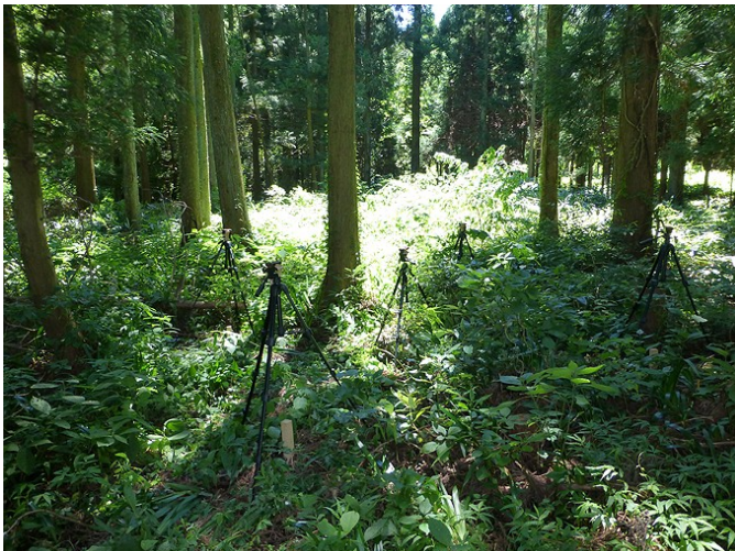
Figure 1: GPS measurements with the crisscross arrangement of the five GPS receivers
