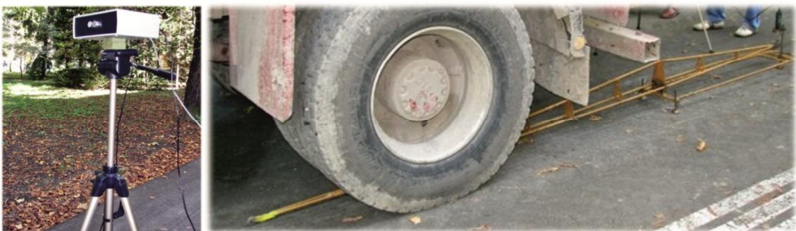
Figure 2: The central data logging unit with the sonar sensor and one Benkelman beam with digital gauge
