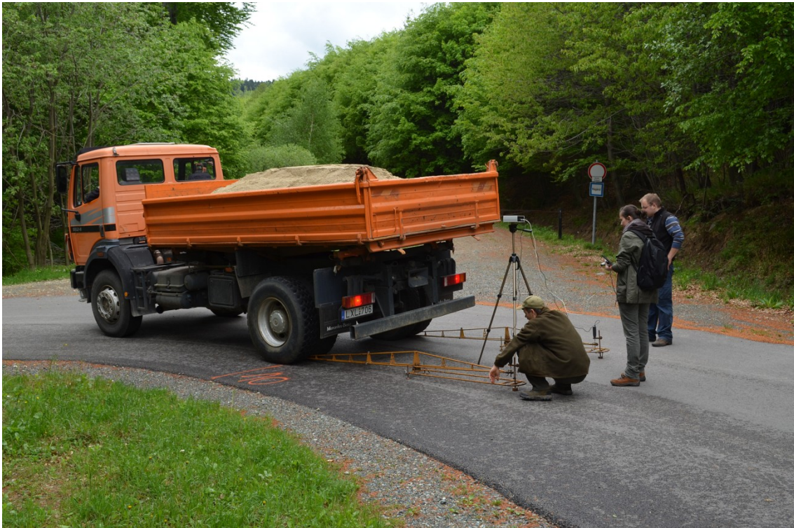
Figure 3: The Advanced Benkelman Beam Apparatus in action
