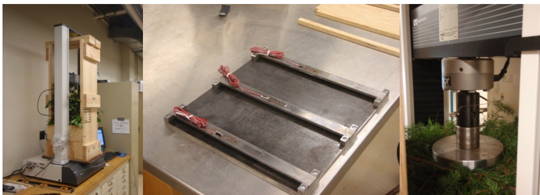
Figure 4: A) Instron testing machine with load box, B) Three strain gauges at the bottom of the load box, C) Loading piston with disc
