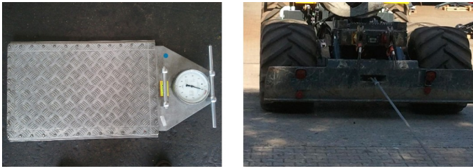
Figure 1: Weighing platform and fixed machine for traction force measurement
