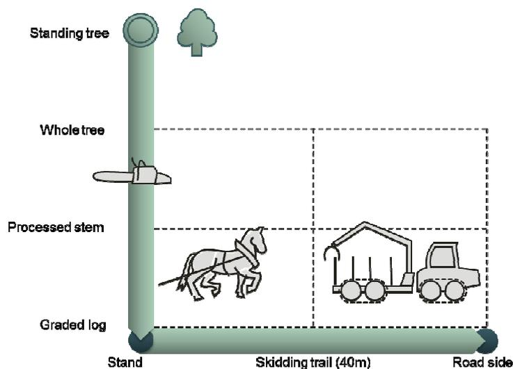
Figure 2: Functiogram of the motormanual felling and horse skidding
