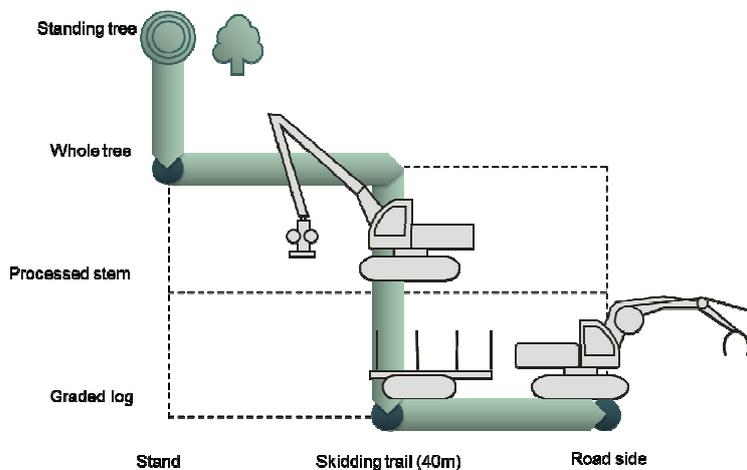
Figure 5: Functigram of the mechanized felling and processing by tracked harvester
