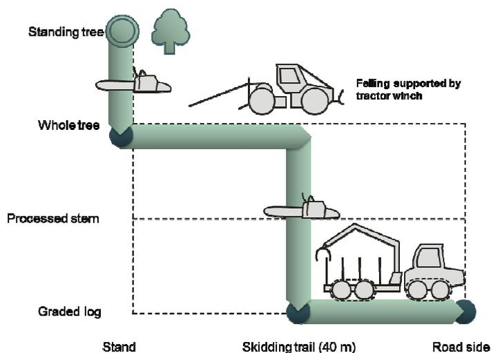
Figure 3: Functiogram of the motor-manual felling supported by tractor winch
