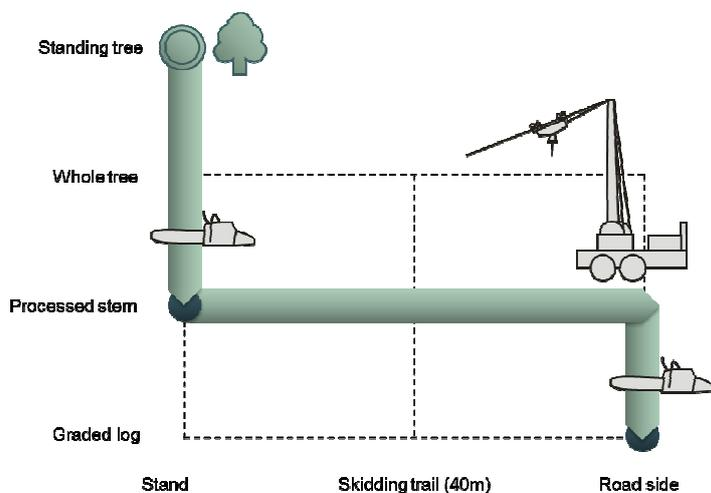
Figure 4: Functiogram of the motor-manual felling and skidding by wire crane system
