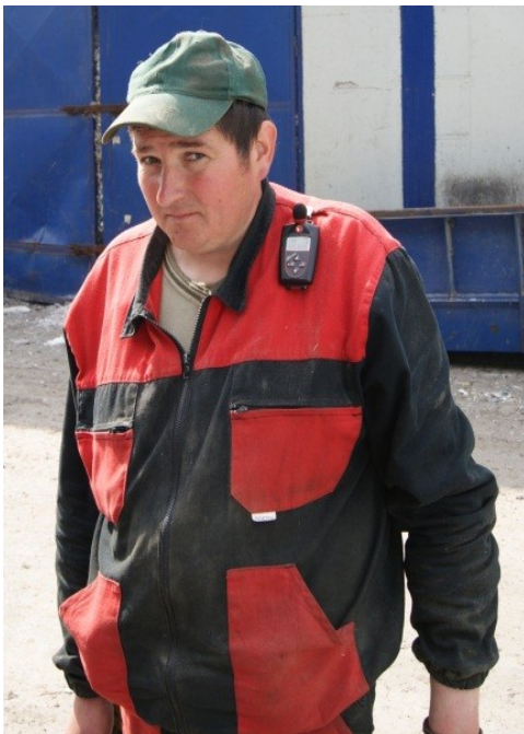
Figure 2: Noise dose meter on the operator
