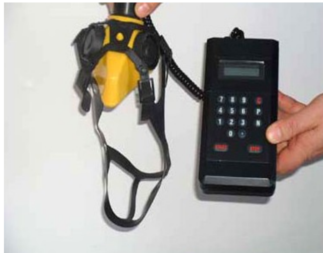
Figure 3: The MWE-1 device for ventilation assessment
