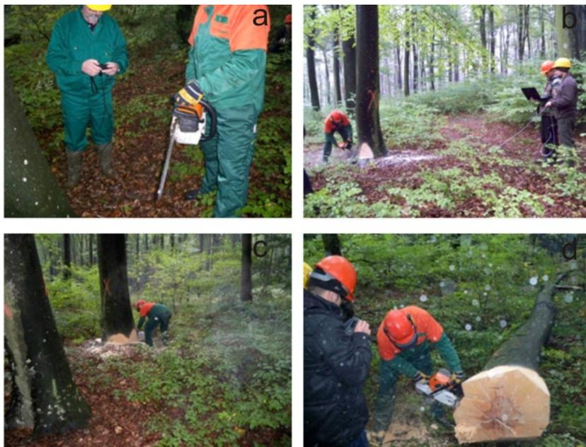
**Figure 2: Some activities during handling the chain saw: a) at idling, b) preparing to turn down, c) turning down, d) cross cutting**
