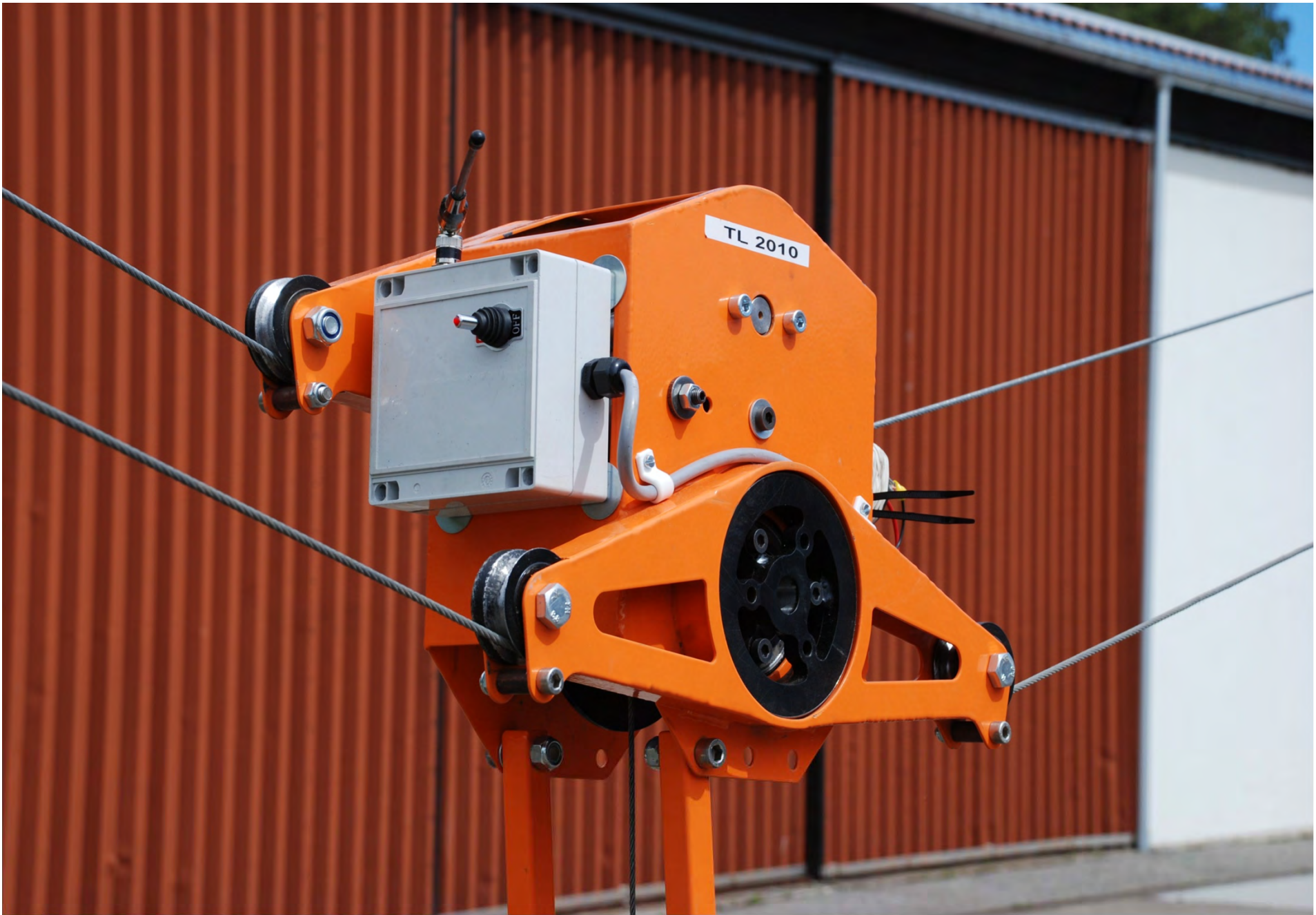
1:3 scale mechanical slack-pulling carriage undergoing testing
