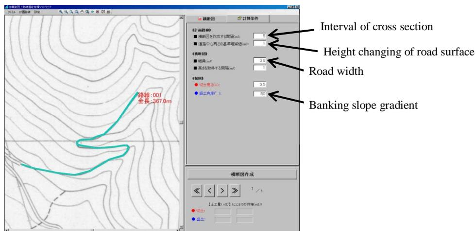
Figure 2: Gauge parameter input window of the software
