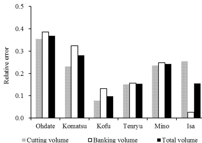
**Figure 4: Relative error of cutting, banking, and total volume**
