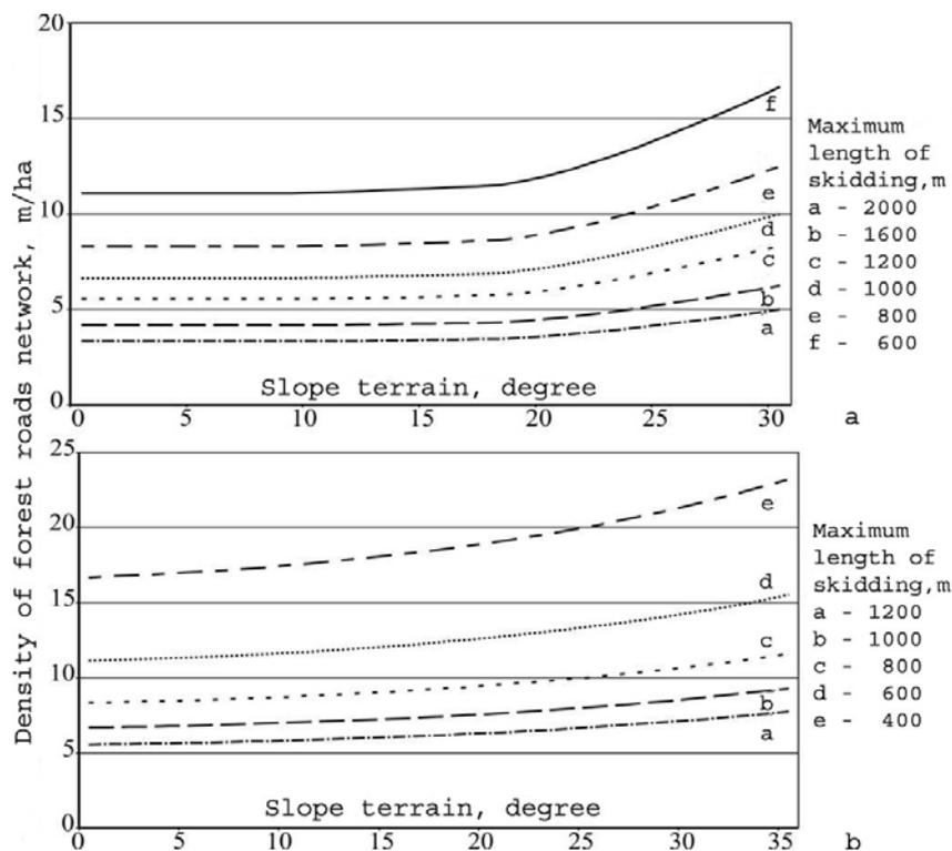
**Figure 2: Dependence forest road network density from slope terrain, where skidding perform by: a – wheeled skidder; b –cable crane**
