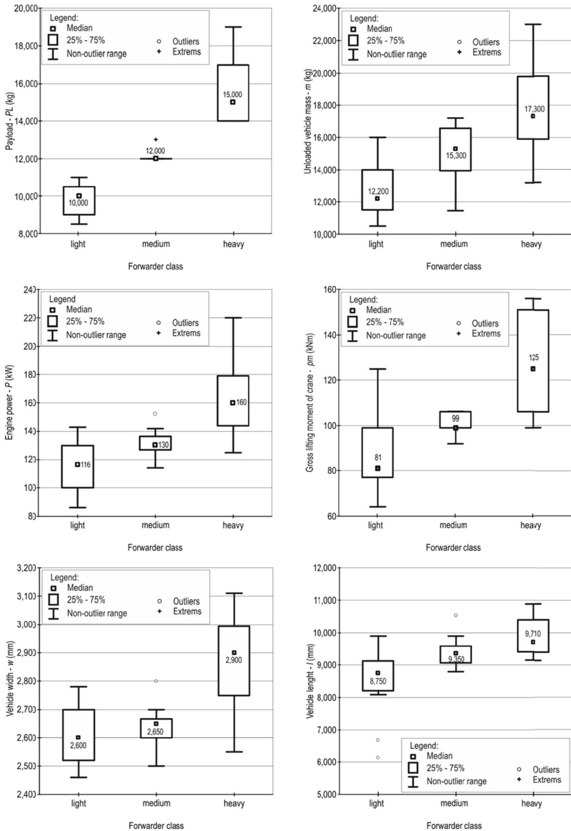
Figure 3: Some of the technical features according to forwarder class
