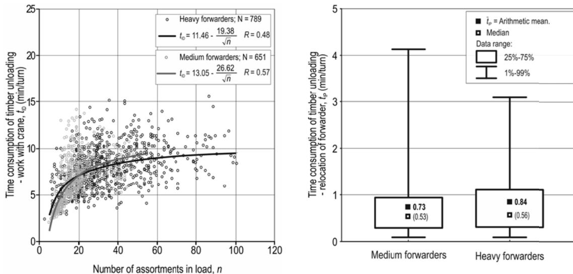
Figure 7: Time consumption of timber unloading
