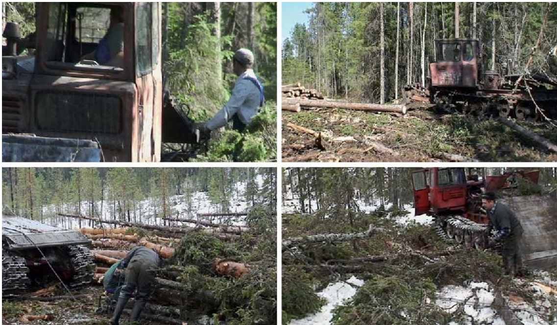
Figure 9: Uncomfortable body positions during operations with a cable skidder
