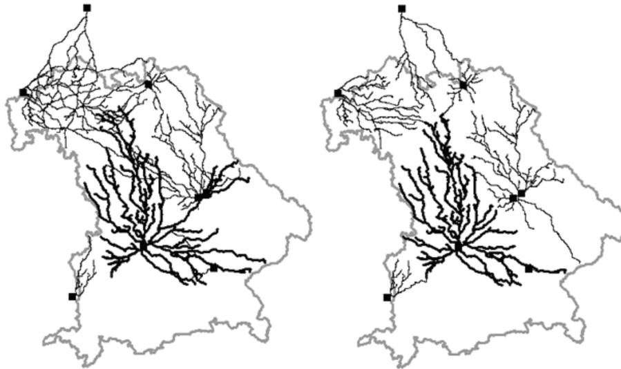
**Figure 2: Assortment: pallet pine. Routes after traditional planning (left) and routes after optimization (right), routes to the mills black, to one mill bold black, country border grey.**
