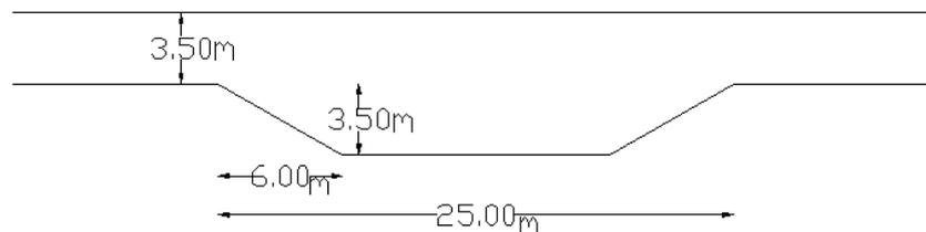
**Figure 4: Proposed Widening along a straight part of a main road to accommodate two-way passing of fire trucks**
