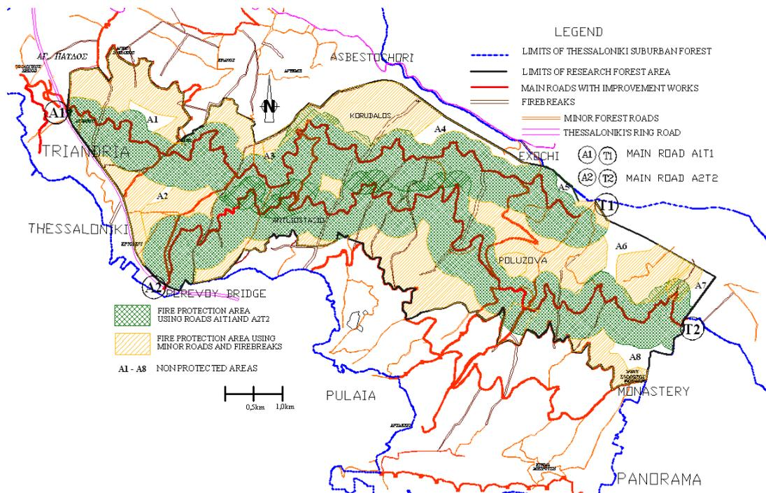
Figure 4: Area of fire protection using a range of 150-300m from forest roads within the research area. (Psilovikos T. 2010)
