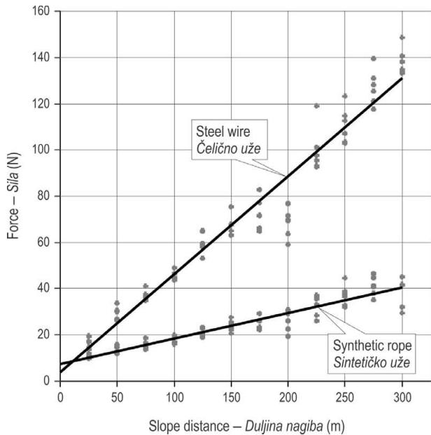
**Fig. 3a** The tensile force exerted on the subject for the steel wire and synthetic rope, respectively. The resistance in the drum of the steel cable was higher than for the synthetic rope at 0 m despite the linear regression indicating otherwise
