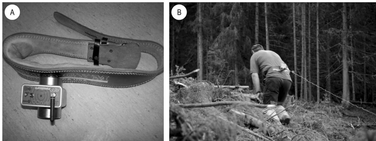
**Fig. 2** Illustration of the belt, dynamometer (A) and steel strawline being pulled out (B)
