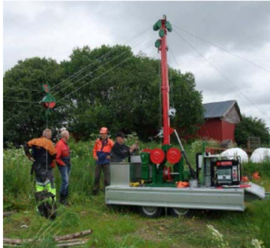
Figure 1: The trailer mounted Owren mini 400 yarder
