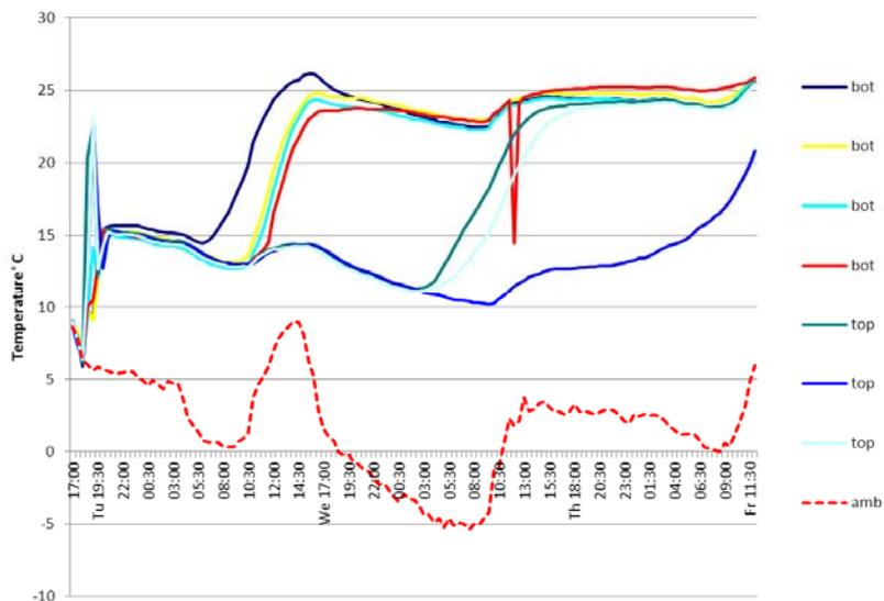
**Figure 2: The air temperature at the bottom and top of the container and outside the container.**
