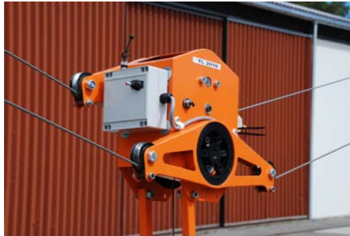
Figure 3 The completed 1:3 scale mechanical slackpulling carriage undergoing testing
