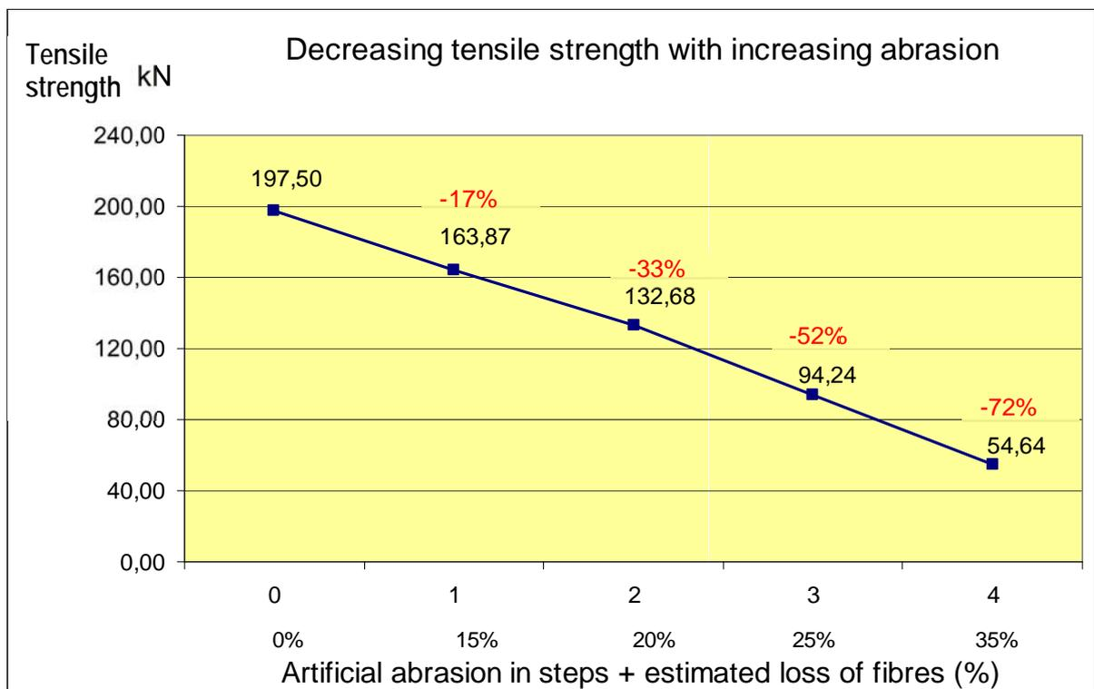
**Figure 5:** Loss of tensile strength with progressive abrasion at four abrasion levels departing from the unused rope (Level 0)
