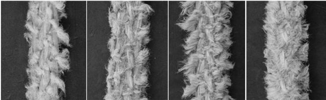
**Figure 1 to 4:** left to right, four levels of progressive artificial abrasion– it is hardly possible to distinguish the individual levels from their surface structure.
