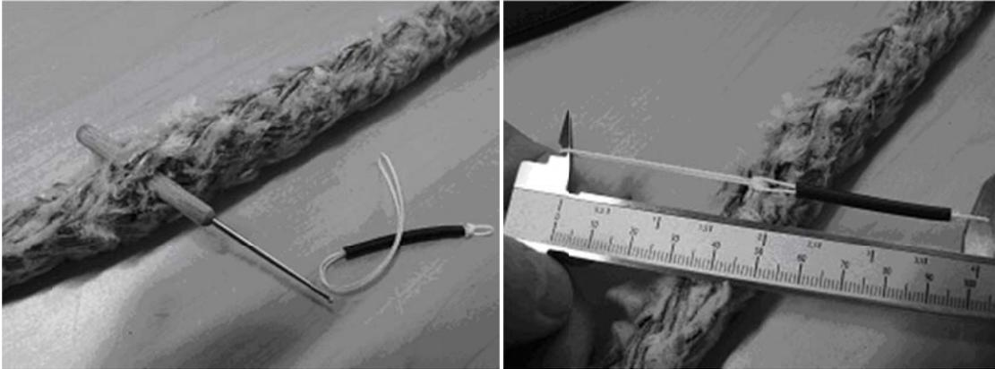
**Fig. 8 & 9: Identification of profile loss by measuring the individual strands**
