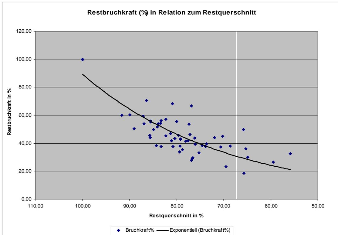
**Figure 10: Remaining breaking strength (%) in relation to remaining profile (%) – all rope products**
