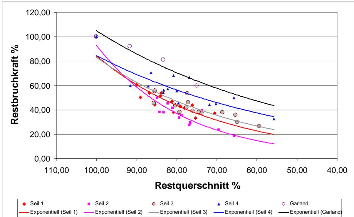
**Figure 11: The remaining breaking force (%) in relation to the remaining profile (%) – according to rope type, supplemented by the above mentioned results from the laboratory tests by Garland et al.**
