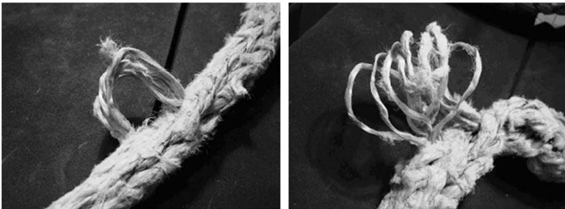
**Figure 6 & 7: The identification of the fibre loss by assessing the monofilaments of the separated strands caused a remarkable disaggregation of the rope**
