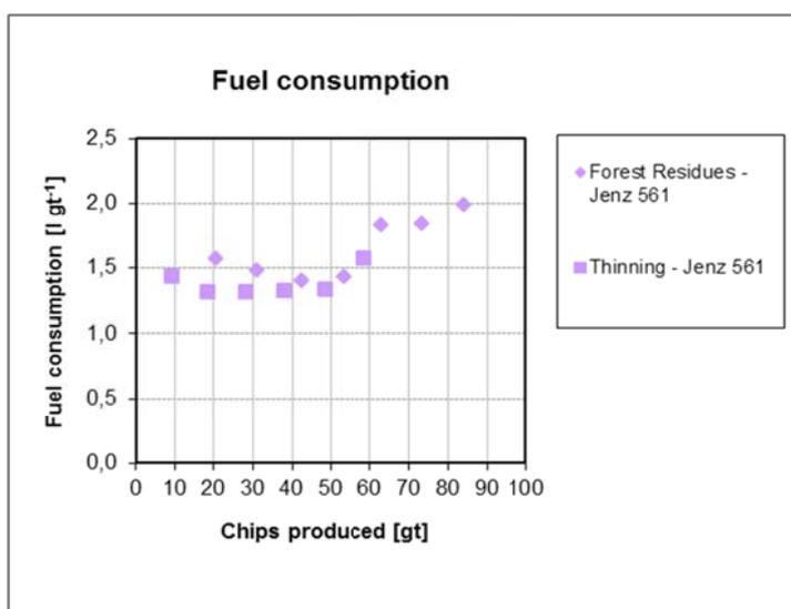
**Fig. 4. Fuel consumption in relation to progressive dullness of drum chipper blades**
