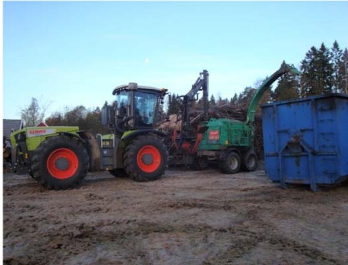
**Figure 1: Chipping of forest residues at a roadside landing located in Skultorp**
