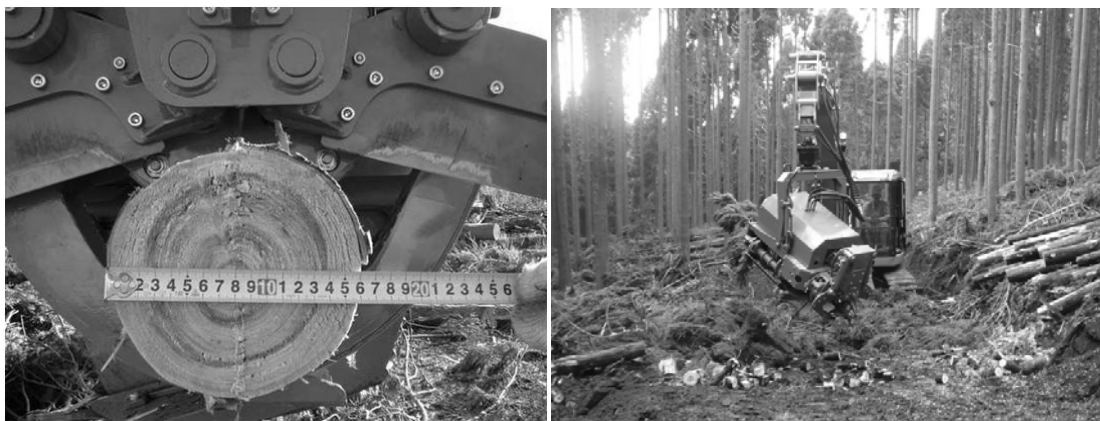
Figure 1: Processor with chopping equipment and the cutting surface of a top
