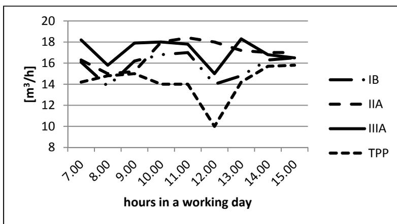
**Figure 2: Work productivity rate of BANDIT 2090 in particular working hours**
