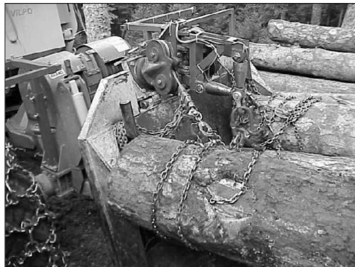
Figure 5: Measurement of pulling force in the winch wire rope
