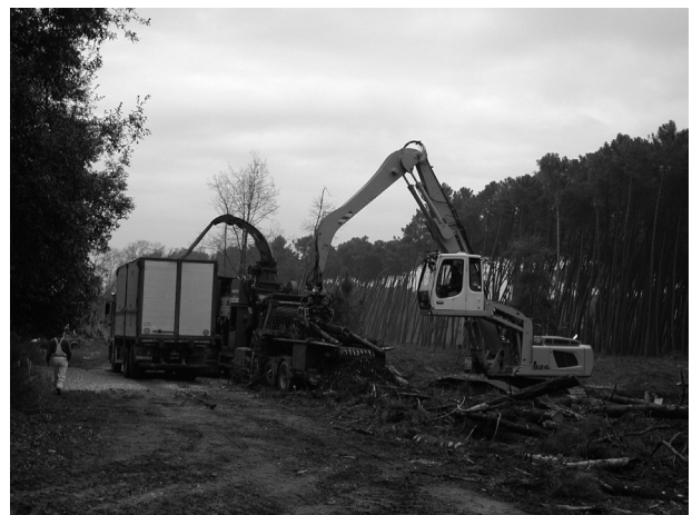
Fig. 2 Roadside chipping operation: the heavy chipper filling a chip van Slika 2. Iveranje na stovarištu: teški iverač puni kamion iverom
