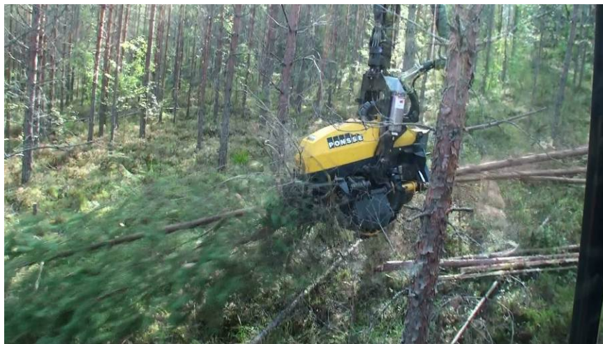
Figure 4: Software-based multi-tree cutting of roundwood-sized timber with a Ponsse H7 harvester head, as viewed from a Ponsse Fox cab
