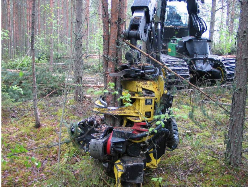
Figure 3: The John Deere H412 multi-tree harvester head in action in pulpwood thinning
