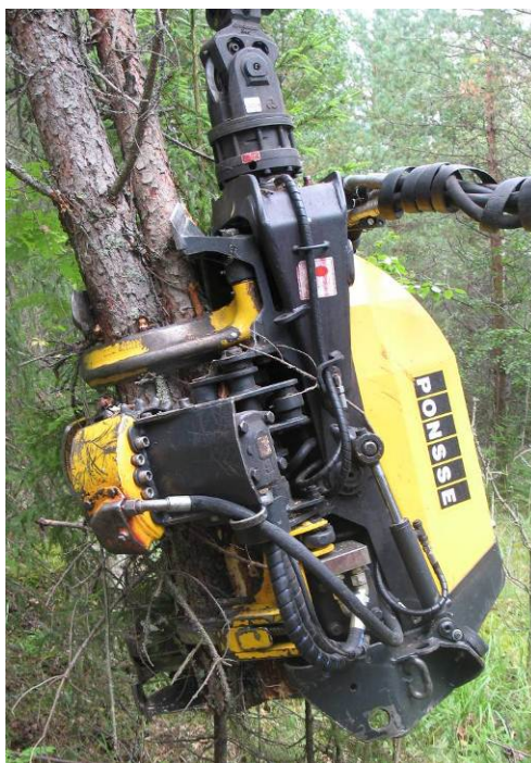
Figure 2: The Ponsse H53e harvester head with a multiple-tree processing property.
