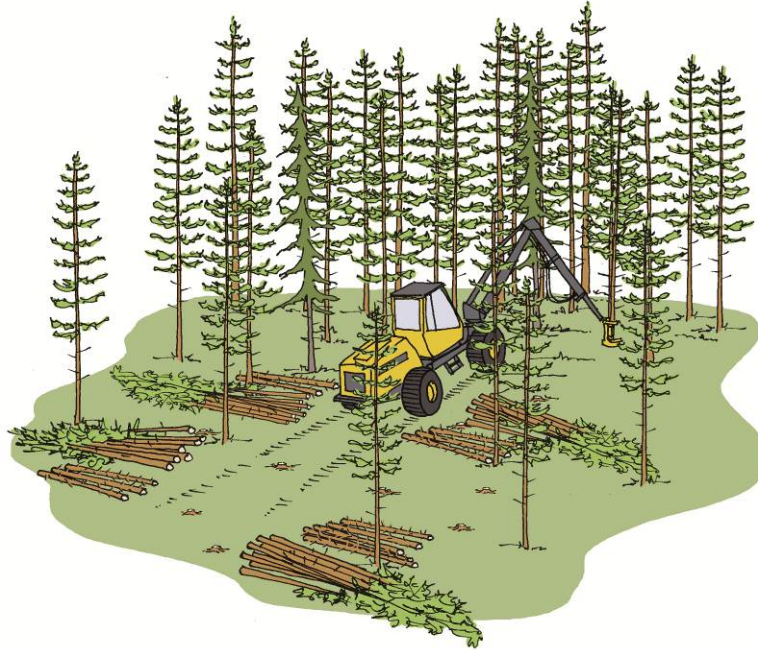
Figure 1: The integrated wood procurement system based on the two-pile method, in which pulpwood and energy wood fractions are stacked into separate piles in early thinnings.
