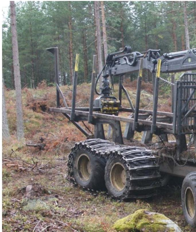
**Figure 1: The load area on the forwarder. Note the framework on the bunks and the rearward extension with the two slightly rearward leaning additional rear posts.**
