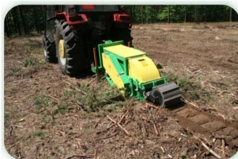
Figure 3: Principle of Milling ( http://www.otljarocin.lasy.gov.pl )
