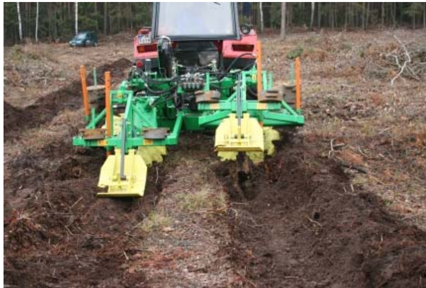
Figure 6. Classical forest active disk plough ( http://www.otljarocin.lasy.gov.pl )
