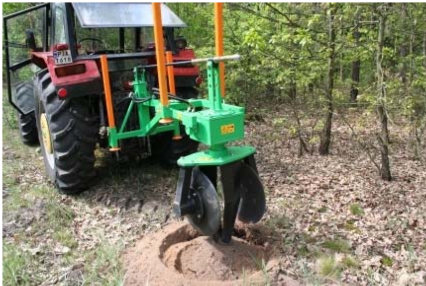
Figure 4: Principle of Forest soil drilling ( http://www.otljarocin.lasy.gov.pl )
