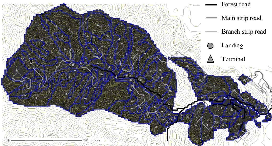
Figure 3: Road network with main strip roads on ridges and branch strip roads at 100-m intervals
