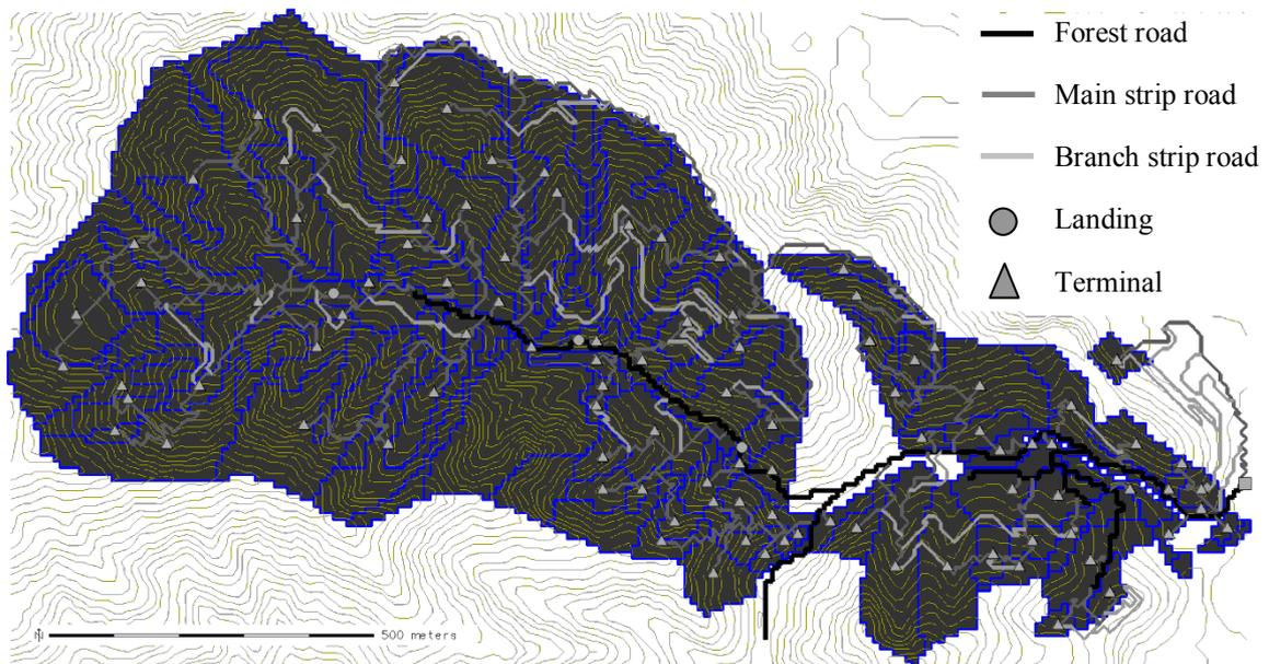
**Figure 4: Optimized road network with main strip roads on ridges and branch strip roads at 100-m intervals**
