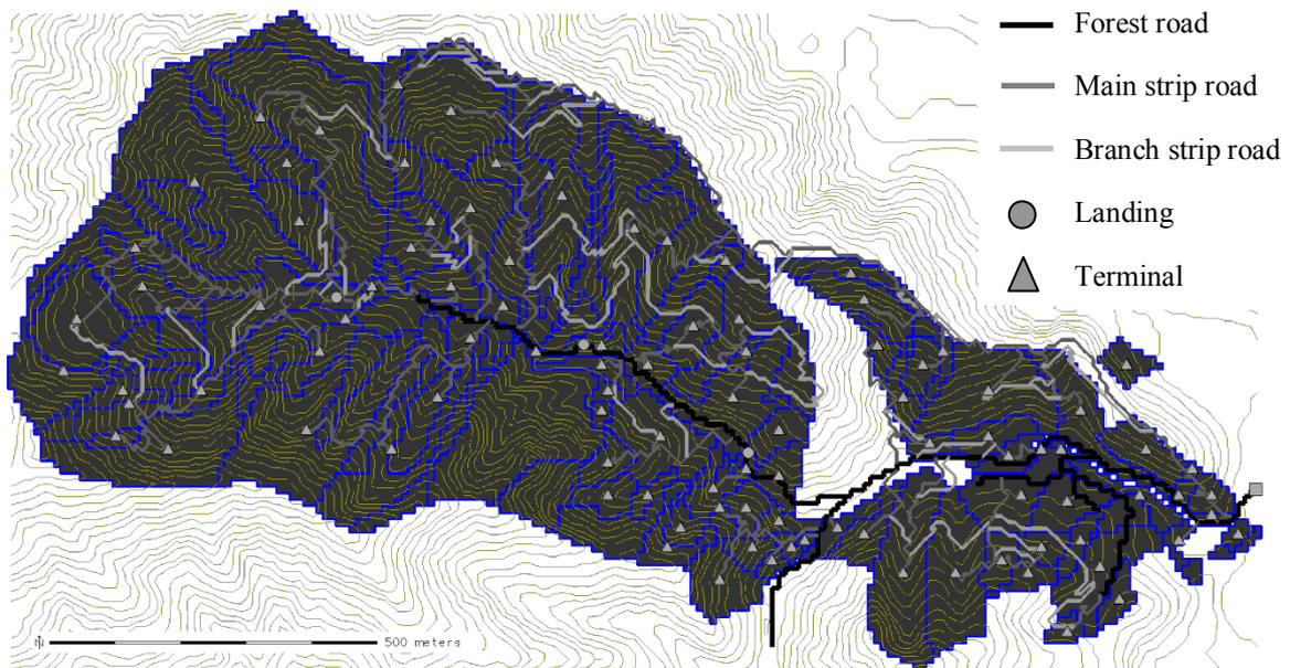
**Figure 5: Optimized road network with 70 attainment points on main strip roads on ridges and branch strip roads at 100-m intervals**
