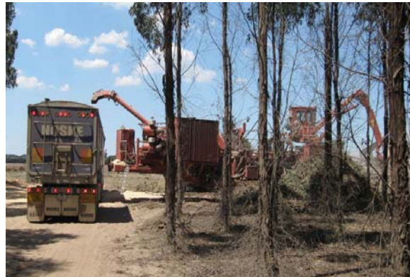
Figure 2: Chip-van truck in in-field chipping operation
