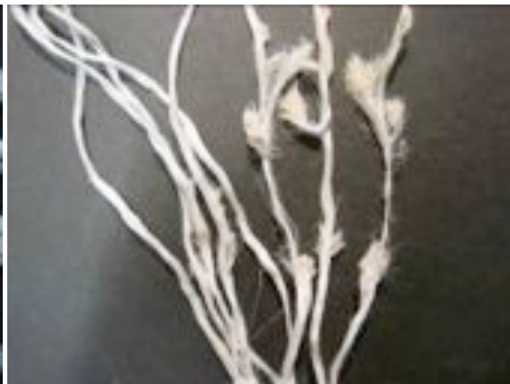
Figure 13. The loss of fibres could be estimated at the individual yarns of the strand
