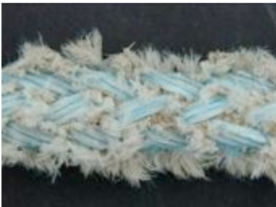
Figures 9. The surface of two test ropes after 40 trips
