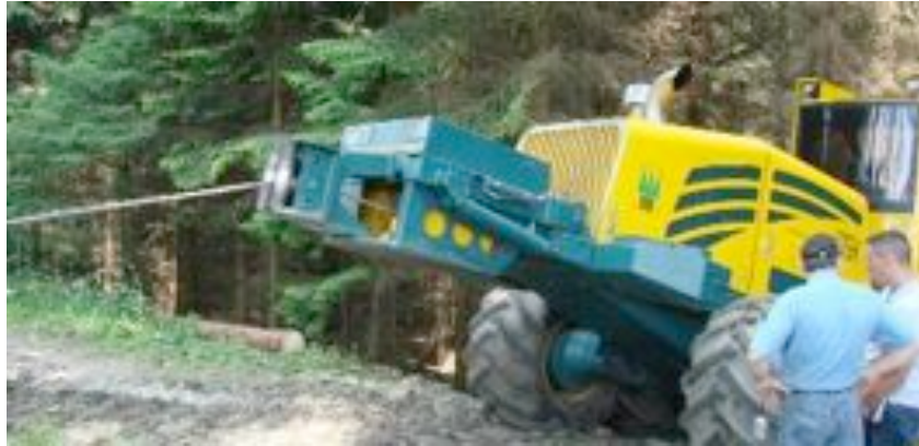
Figure 11. Harvester hanging in a steep slope on a rope in condition similar to the test ropes on figure 9
