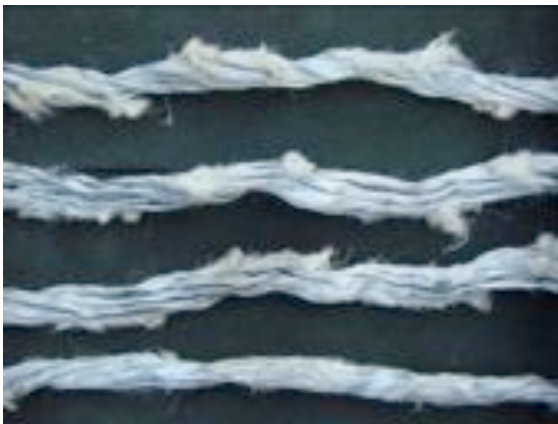
Figure 12. Strands from 4 differently worn ropes
