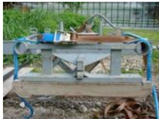
Figure 3. The test rope is fastened on the skid
