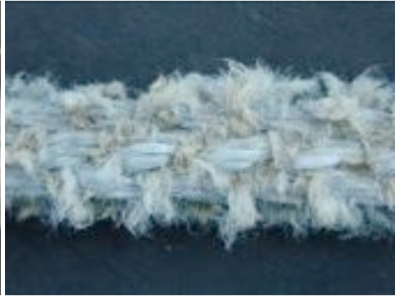
Figure 6. The reference rope after 20 trips
