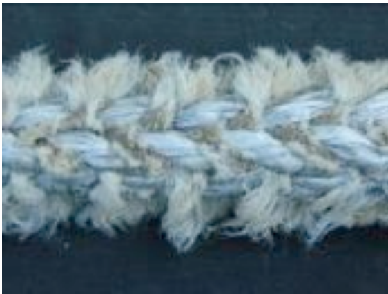
Figures 7. The reference rope after 30 trips
