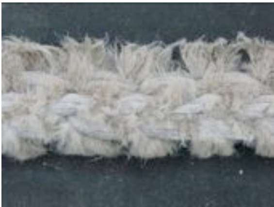
Figure 8. The reference rope after 40 trips
