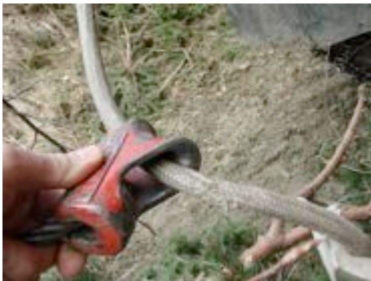
Figure 1. Abraded area on a coated synthetic rope
