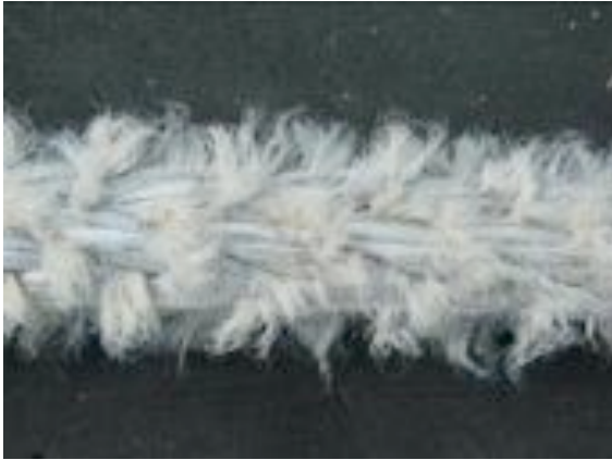
Figures 5. The reference rope after 10 trips
