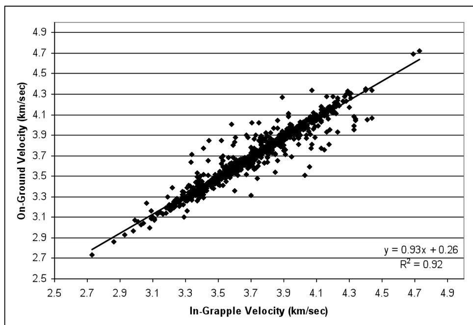
**Figure 1.** Relationship between acoustic velocities in the grip of a harvester/loader grapple and those on the ground with no contact to harvesting equipment.
