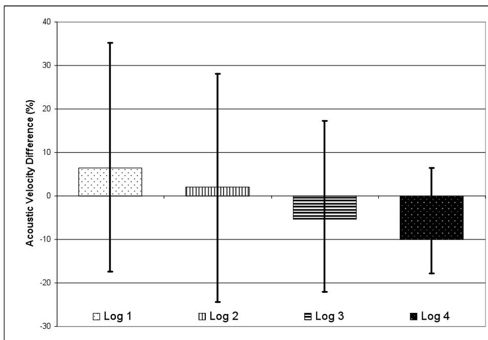
**Figure 2.** Average percent difference between whole tree acoustic velocities and those measured on each subsequent log produced from that tree. The “error bars” represent the range in percent difference for each log
