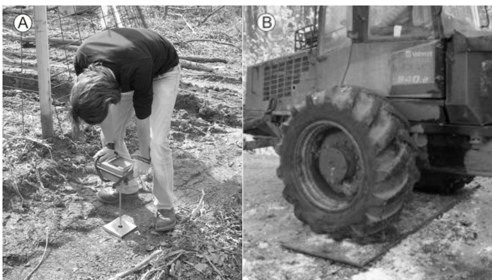
Figure 1. Cone index measuring and weighing of forwarder front axle at the platform with axle scales
