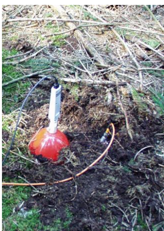
Figure 1 Probe with cover for measuring of CO 2 efflux (red), probe for CO 2 concentration in soil air on right
