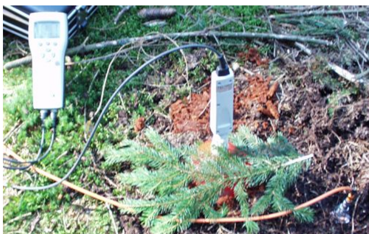
Figure 2 Measuring instruments CARBOCAP GSM70 with measuring probes of CO 2 efflux from soil and CO 2 concentration in soil air on control plot
