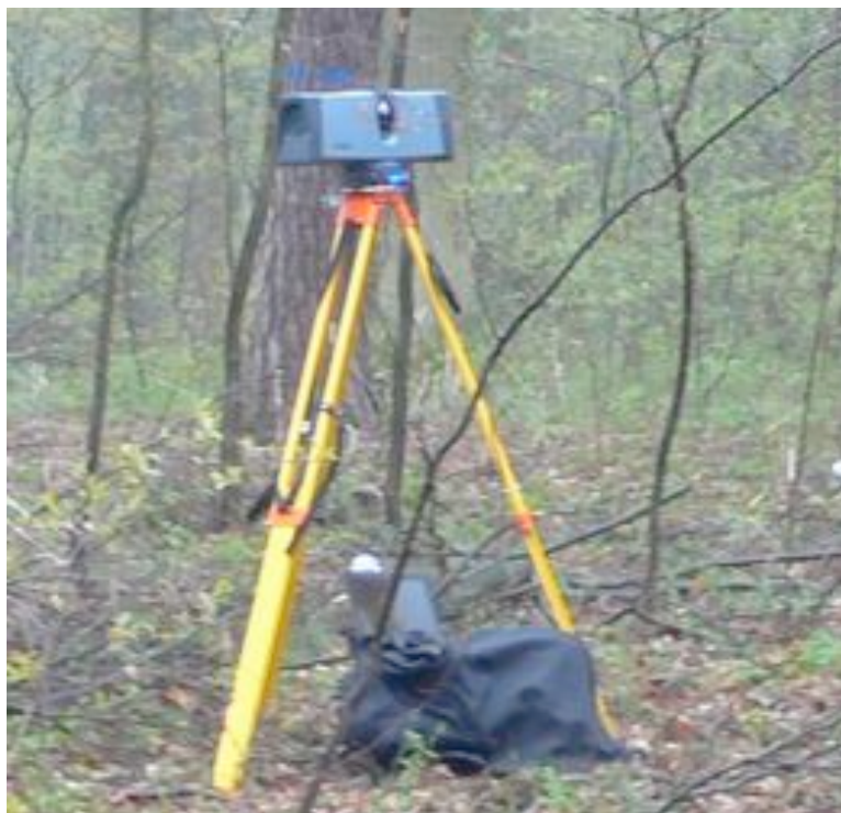
Fig. 4 Trimble terrestrial laser scanner CX 3D
