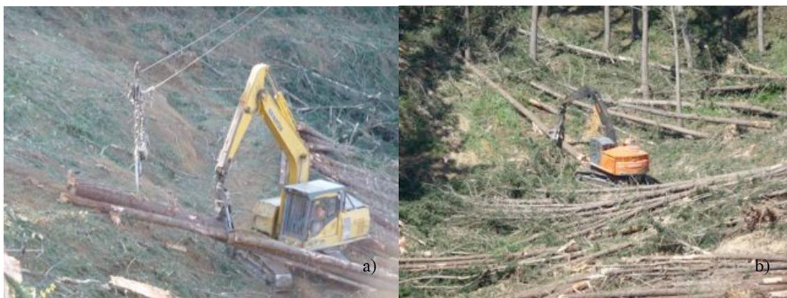
**Figure 3.** a) Bunching excavator presenting load for grapple yarder extraction (Wood Contracting Ltd.) and b) Felling and bunching on broken terrain at the bottom of a slope (Kelly Logging Ltd.).
