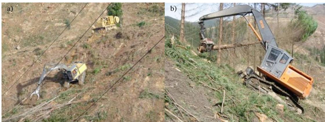
**Figure 1.** a) An excavator attached to a winch mounted on a bulldozer (Wood Contracting Ltd ) and b) An excavator, with integrated winch, attached to a stump (Kelly Logging Ltd).
