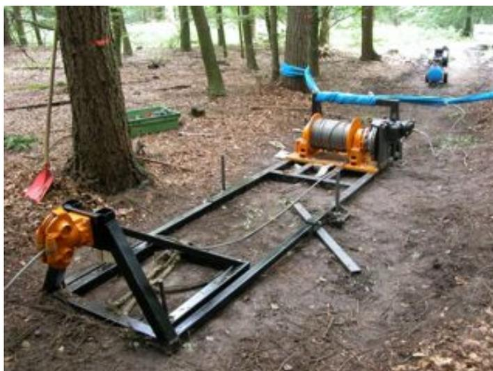
**Figure 1.** Deceleration machine installed on a skidding lane
