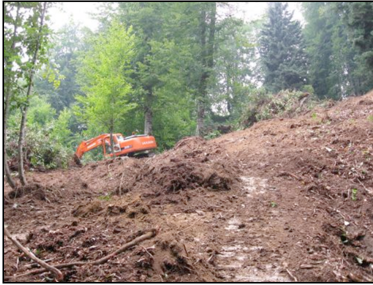
Figure 4. The use the excavators in clearing of Rhododendron spp. activities (Duzce, Turkey)
